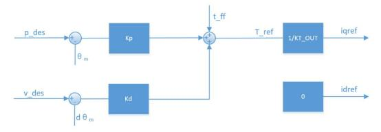
Derived Control Modes from MIT Mode Based on MIT mode, multiple control modes can be derived:
